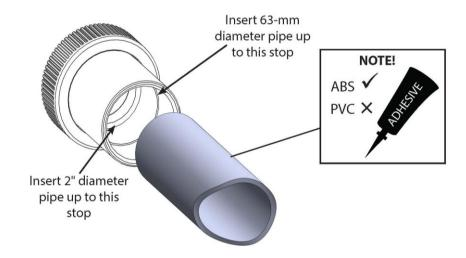
For pipework 50-mm or 1<sup>1</sup>/<sub>2</sub>" in diameter.
