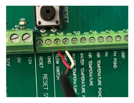
Water temp sensor (does not matter what way round the wires go)
