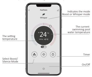
2. For heat pump with Heating and Cooling function:
