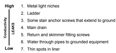
To use the LeakTrac 2400 most effectively it is necessary to create the strongest possible "Leak Track going to the leak, while eliminating or disregarding other connections to ground that are not leaks.
