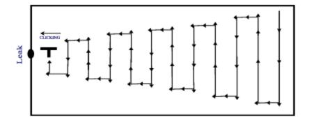
Most leaks are discovered as you are moving the probe in the direction producing a whine then all of a sudden the signal stops. This indicates that the probe has passed over the leak and is now pointing away. Turn the probe around and carefully examine the area just passed.
