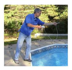
Clip the Probe assembly to the bottom of the telescoping vacuum pole and attach the cord to the side of the pole with tape. Plug the phono plug into the back of the Signal Processing Unit.
